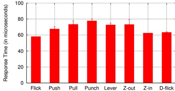
Figure 12: **Response time for various gestures.** The maximum response time is less than  $80 \mu\text{s}$  across all the gestures. Z-in, Z-out, and D-flick refer to the zoom in, zoom out, and double flick gestures.
